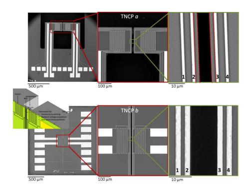
**Above**. The two measurement platforms. Top: TNCP a, cantilever-based design; bottom: TNCP b, membrane-based design. The schematic inset illustrates Platform b's cross-section to show its layout. In both cases, the electrodes are made of Pt.
